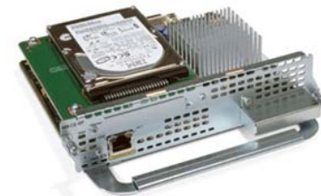
Access Router Module Appliance
